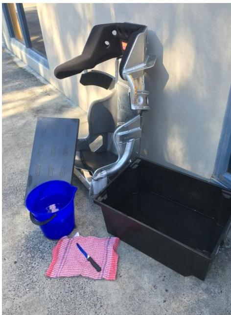
Tools required for pad installation – Pad, SFI sticker, Bucket, Towel, Sharp Blade, Plastic Container, Hot Water
