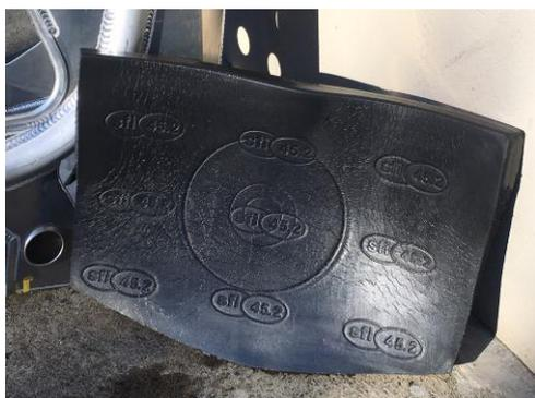
**Step 4** - Once desired shape is obtained remove from seat and allow to dry. Note: water may leak from unsealed cuts.
