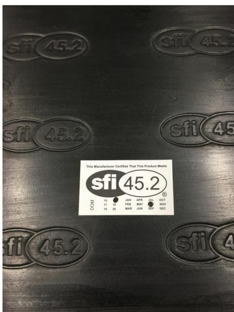
**NOTE:** If the padding is to have a glued Nomex cover ensure the SFI sticker is able to be seen by a scrutineer i.e. ensure sticker is on the underside of the pad.
